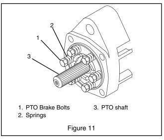
**NOTE:** Do not tighten the bolts in a circular sequence, that is, by tightening the bolt next to one which was just tightened. The bolts should be tightened in a cross sequence, that is, by tightening one bolt, then tightening the bolt which is across from it on the plate. Continue tightening the bolts in this sequence until all the bolts are tightened.
